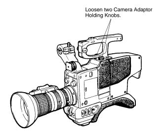
1-2 Tighten two Camera Adaptor Holding Screw/knob(2) firmly and make sure the adopter is securely fixed to the camera.
